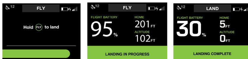
Figure 4.3.2.1: Controller - User-Initiated Landing
