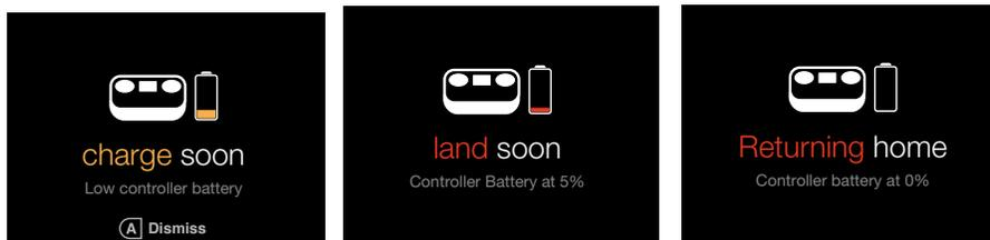
Figure 6.2.6.1: Controller - Controller Battery Alerts
