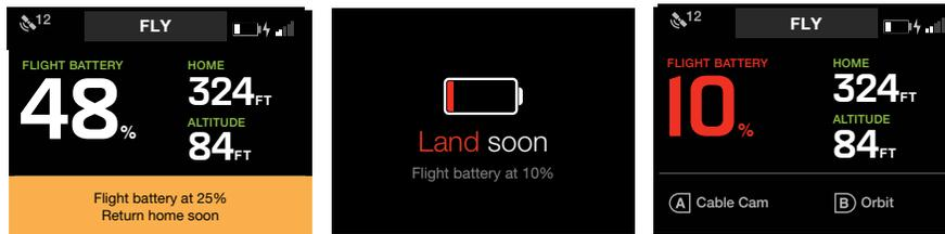
Figure 6.2.5.1: Controller - Low Battery Alerts
