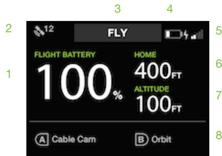
Figure 4.5.2.1: Controller In-Flight Data Display
