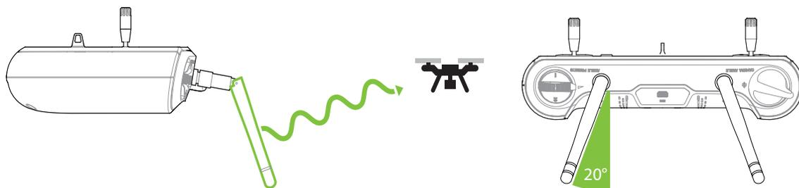
Figure 3.11.5.1: Controller Antenna Orientation
