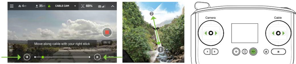
Figure 5.2.2.1: Cable Cam Controls
