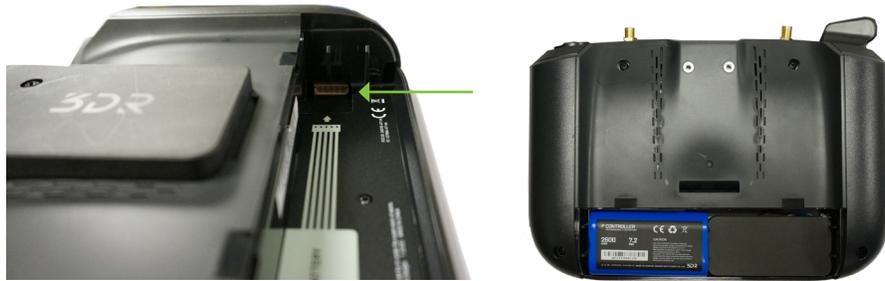
Figure 7.1.6.1: Controller Battery Installation
