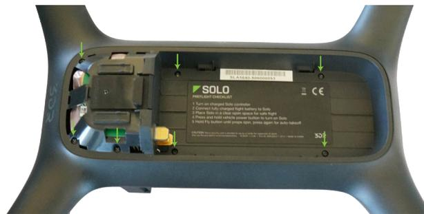
Figure 7.5.2.1: Battery Tray Removal
