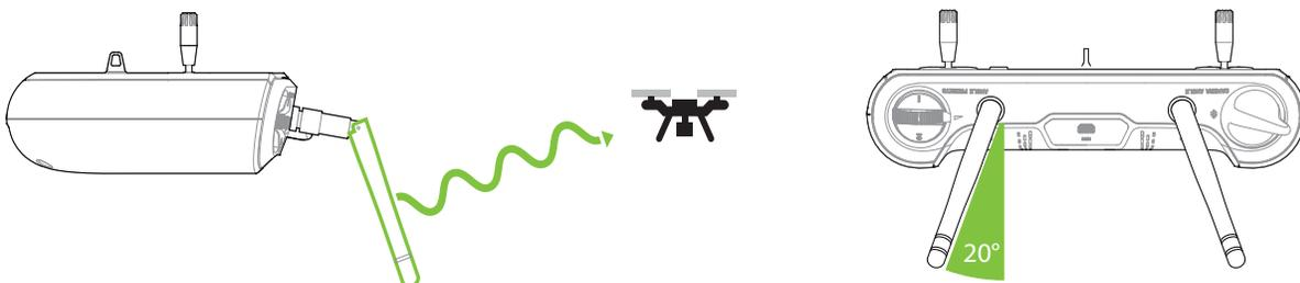
Figure 3.12.5.1: Controller Antenna Orientation
