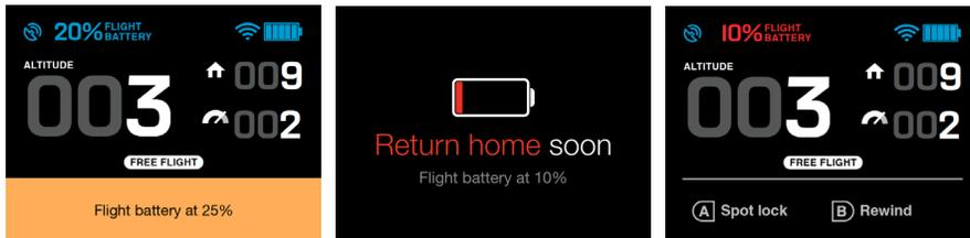
Figure 6.2.5.1: Controller - Low Battery Alerts
